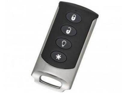
Description: A durable, pocket-sized, wireless device that allows the system user to conveniently operate security and smart home systems. Easy to use, Keyfob gives the user the ability to remotely arm and disarm the system, and activate auxiliary panic alarms.
